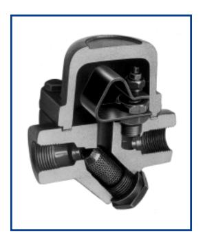
A series of steam traps incorporating integral check valves and Y-type strainers for energy efficient operation on services up to 200 psi. Designed to handle the varying loads of process applications and provide fast start-up and modulating discharge with no live steam loss.
