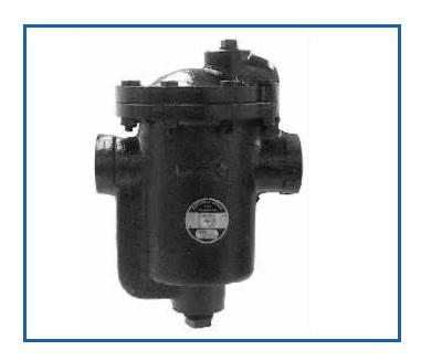
Bestobell's IB18H Series steam traps are horizontal type bucket traps featuring a side inlet and side outlet. They are ideal for general steam service and feature a heavy-duty cast iron body and stainless steel bucket for long-term operation and reliability. For process, heating, and dripleg services with pressures to 250 psig (17.2 bar). Available in 1/2" through 2-1/2" sizes.
