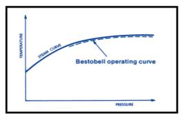
Following the steam curve is the key to efficient steam trap performance. Utilizing dual thermostatic/thermodynamic forces allows Bestobell delta traps to match the steam curve, meaning that the energy in the steam is efficiently used by the process and not wasted in operating the trap.
