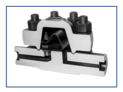
An excellent choice for high pressure steam main dripleg service on low to medium load applications with differential pressures as high as 2,000 psi. Fast start-up, and reliable operation with no live steam loss.
